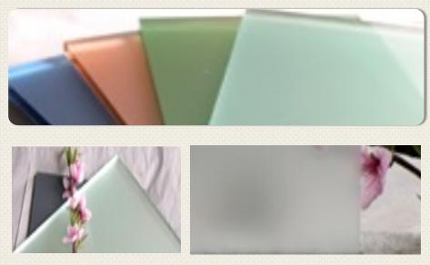
SGC Acid-etched Glass is manufactured with quality clear float glass, low iron glass and tinted float glass. The acid is applied to one surface or tow surfaces of the glass to create a smooth satin finished surface. It is available with clear and tinted float glass, low iron glass, laminated glass, painted and mirrors. It is available in glass thicknesses from 3mm to 19mm.
